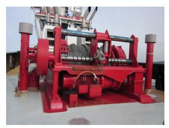
Model MW12 1D80BR: 12t drum winch, spooling, 20m/min, 80t brake
