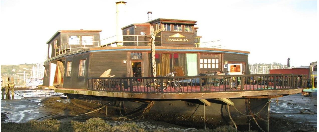
**The Vallejo was originally built in 1890 as a side wheel paddle steamer operating in US waters. The hull was originally riveted plate construction and the superstructure has been extensively modified over the years. From the 1950's onward the vessel was laid up in a tidal mud berth as a house boat, it became well known in the artistic community especially during the 1950-60's beatnik era.**
